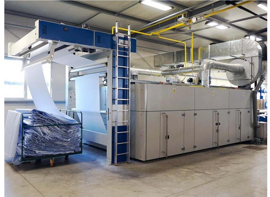
❑ Industrial hot air dryer
